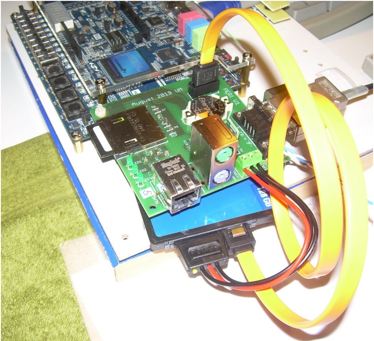
Figure 1 : The power and signal connetions of the SATA drive to the PERI board.
