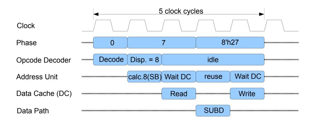
If the data cache is accessed the module DECODER is not active every clock cycle (= idle). The reason for this not ideal behaviour is the virtual memory support. If the cache detects an abort the state of M32632 is reset to the beginning of the instruction. The task of reseting is simplified if the DECODER is waiting for the data cache finishing the current access.
