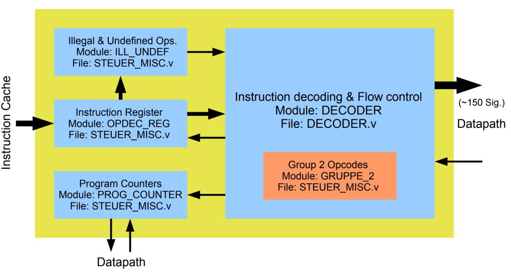
The three most important elements of STEUERUNG are the architecture program counter PC\_ARCHI inside the module PROG\_COUNTER, the register OPREG in the module OPDEC\_REG and the register phase\_reg in the module DECODER.
